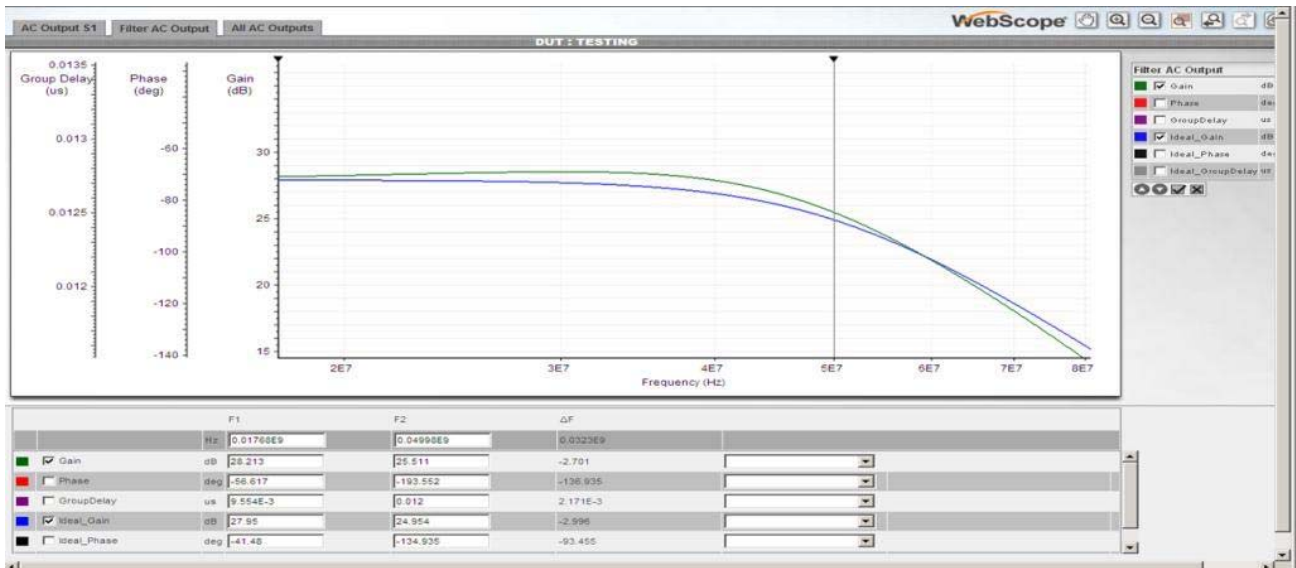
FIGURE 58. COMPARISON OF SIMULATED TO IDEAL GAIN RESPONSE
